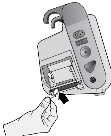
Figure 26-3. Cleaning the Print Head
