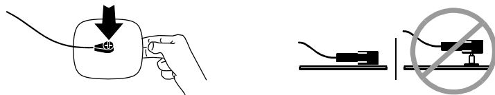
Figure 5-4 Connecting FAST-PATCH Electrodes to Defibrillation Cable
