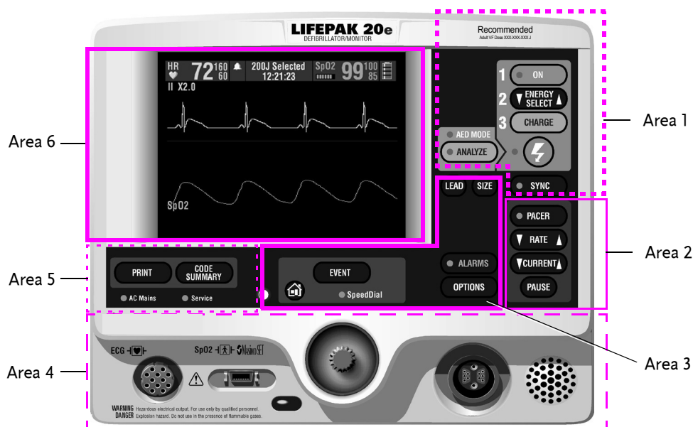
Figure 2-3 Front View without Door
