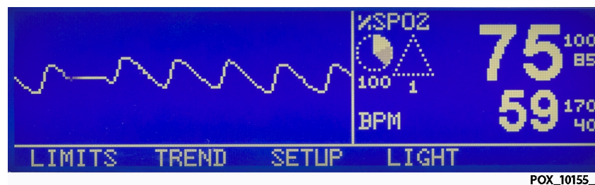
Figure 87. PLETH Display with SRC-MAX tester-generated waveform
