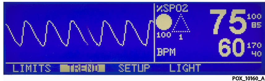
Figure 91. PLETH Display with SRC-MAX increase in modulation
