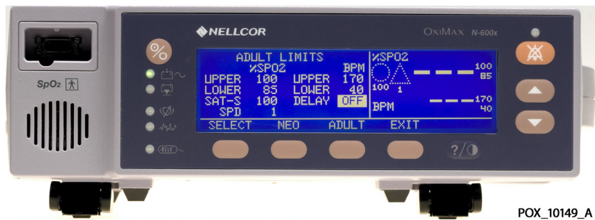
Figure 71. Testing Pulse Rate Delay Thresholds
