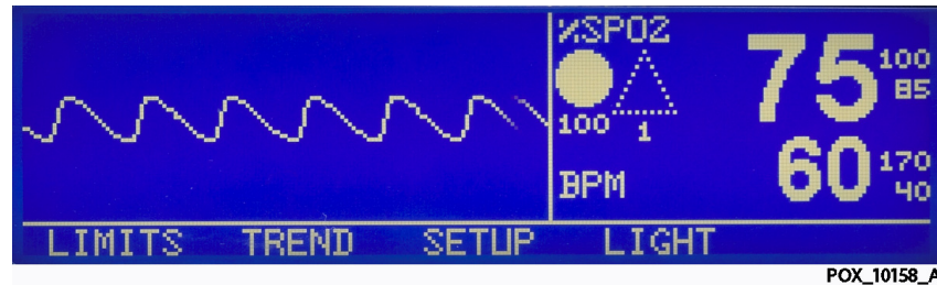
Figure 86. PLETH Display with SRC-MAX decrease to 60 BPM
