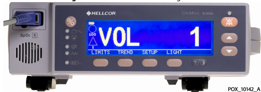
Figure 78. ALARM VOLUME setting of 1
