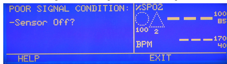
Figure 21. Poor Signal Condition Message
