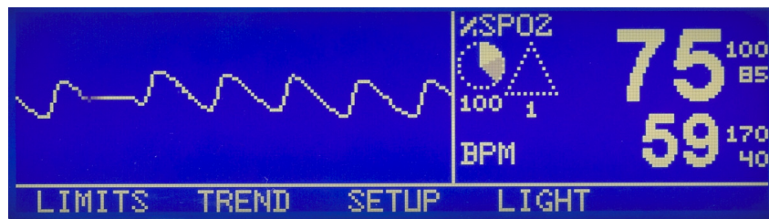
Figure 84. PLETH Display with SRC-MAX tester-generated waveform
