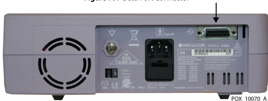
Figure 79. Data Port Connector
