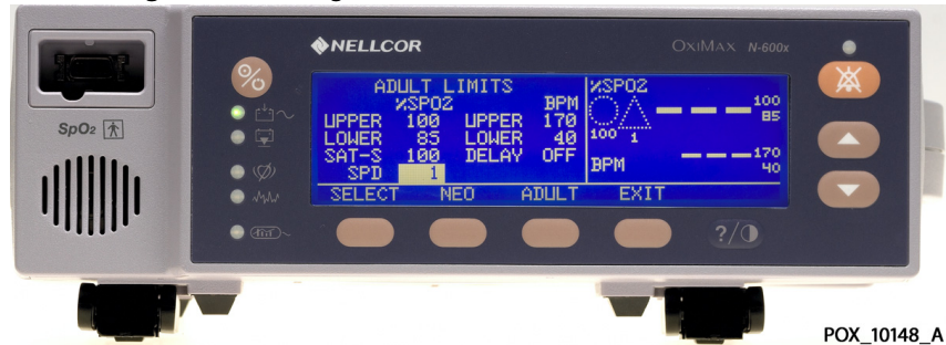
Figure 70. Testing Saturation Pattern Detection Thresholds
