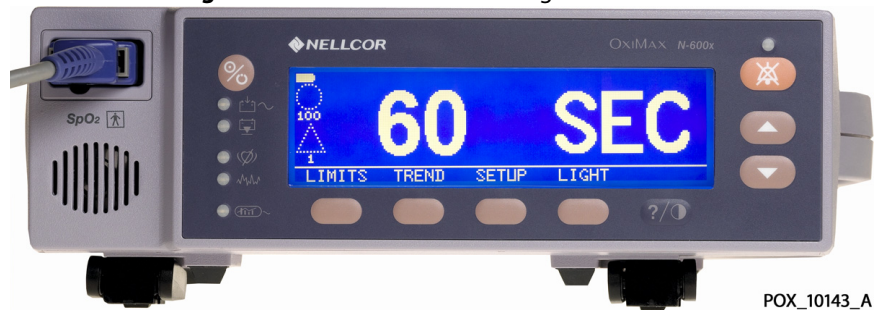
Figure 75. ALARM SILENCE setting of 60 seconds
