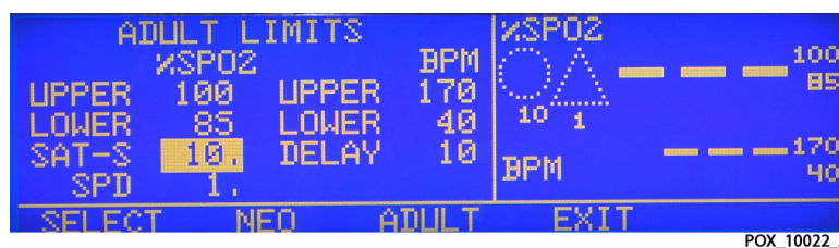
Figure 37. Setting the SatSeconds Alarm Limit
