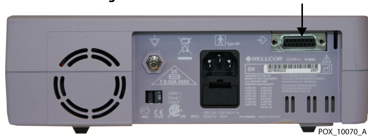
Figure 104. Data Port Connector
