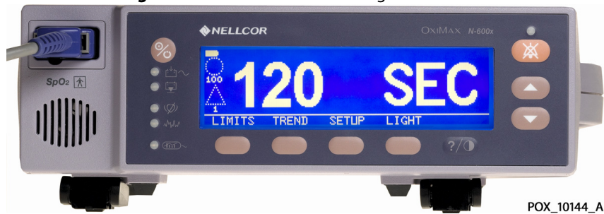
Figure 76. ALARM SILENCE setting of 120 seconds
