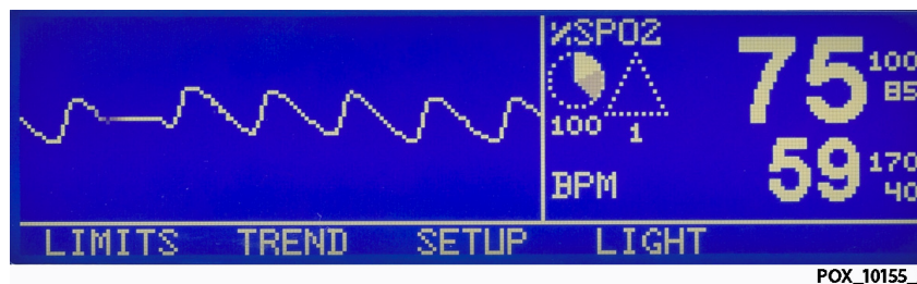
Figure 97. PLETH Display with SRC-MAX tester-generated waveform
