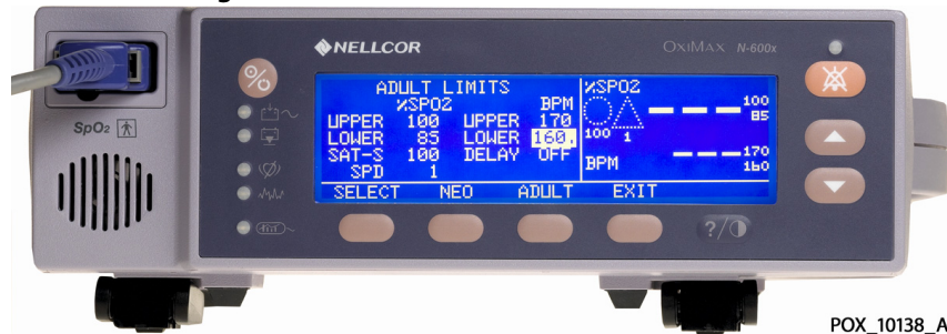
Figure 74. Adult Lower BPM Alarm Limit of 160
