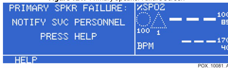
Figure 121. Primary Speaker Failure Screen
