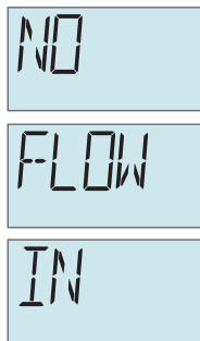
Figure 3-4 NO FLOW IN Alarm
