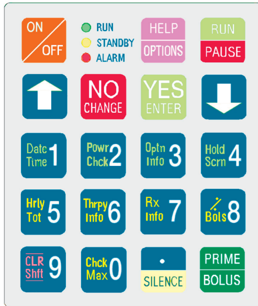
Figure 2.2 IOD Keypad with Info-On-Demand Feature
