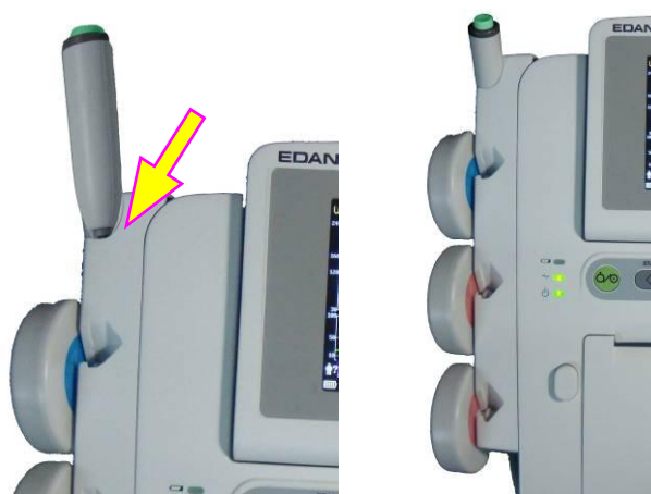
Placing the marker
