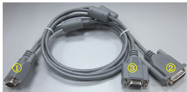
Figure A7-2 Y-shape Signal Cable
