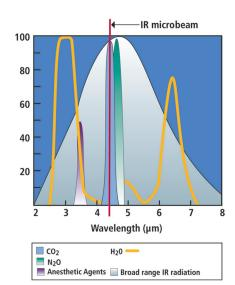
Patented Molecular Correlation Spectroscopy<sup>™</sup> technology uses a highly specific infrared microbeam to provide an accurate measurement of a patient's ventilation.
